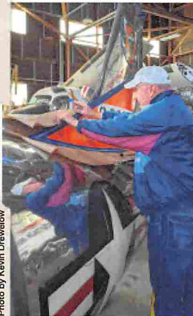
Gene masks the T-33's vertical fin for painting
